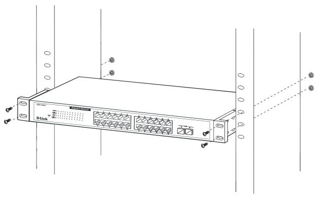
Figure 2- 3. Installing Switch in a rack
